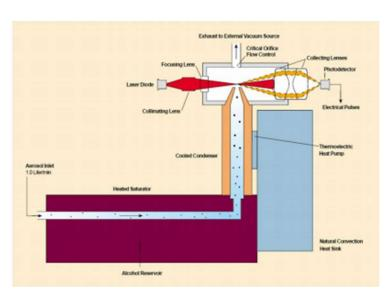
Figure 8: Schema of a condensation particle counter (TSI)
