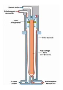
Figure 9: Schema of a differential mobility analyser (TSI)
