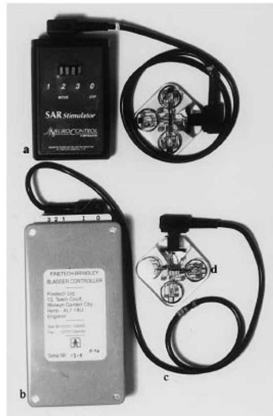
Fig. 2a-d External equipment. a New control box. b Original control box. c Transmitter lead. d Transmitter block
